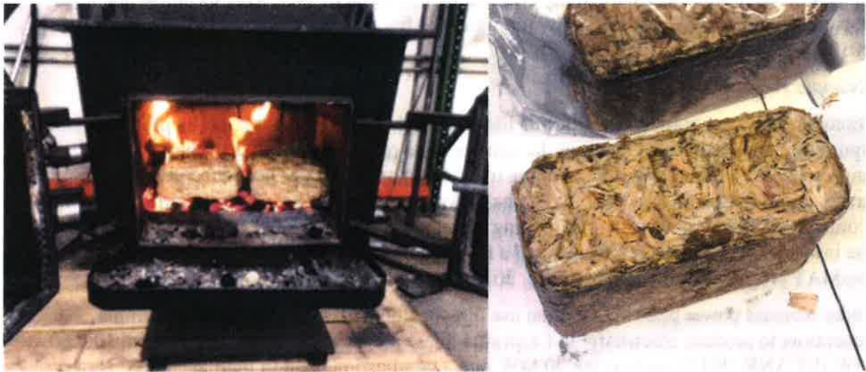
Figure 3. Biomass briquettes burning in a woodstove (left); biomass briquettes produced from tanoak woodchips.
