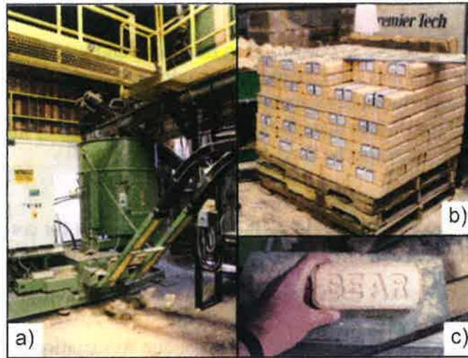
Figure 4. Image a) shows the RUF RB440 installed at Bear Mountain Forest Products, b) shows briquettes produced from the RUF 1100 packaged in groups of six on a pallet, and c) shows an individual briquette produced on the RB440.
